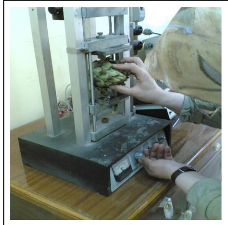
Figure (1): The Stress -Strain tests using an Instron Machine Cole Parmer model (G-08232-28).
