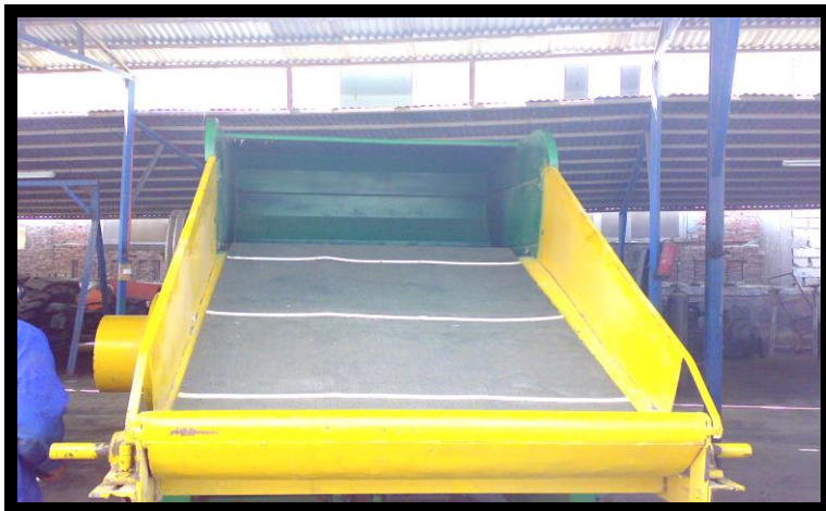
Fig (2): The conveyor belt.
