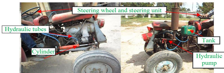
Figure (1): Tractor modifies from mechanical to hydraulic steering
