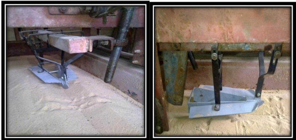
Fig. (2): Developed furrow opener during laboratory tests.
