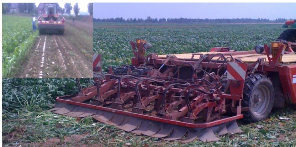
Fig.(1): The BM 300 Grimme defoliator machine with rear attached scalper.
