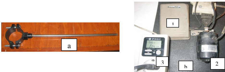
Fig. 3: The arm in Prony brake (a) and (b) the AC N3-70 motor: 1 speed controller 2 and PSGI wattmeter 3.
