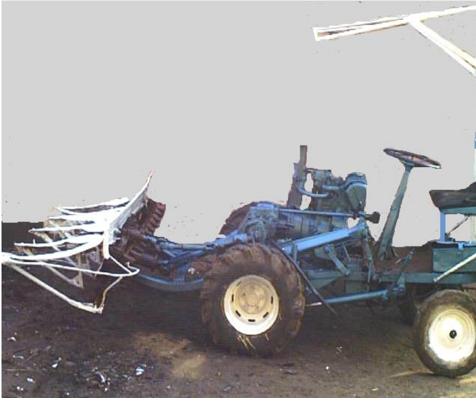
Plate 1:A self propelled vertical conveyor reaper which were manufactured:
