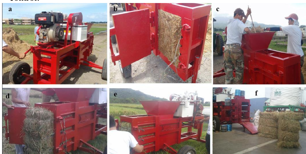
Figure 4: Consecutive testing to enhance the baling mechanism and tying system
