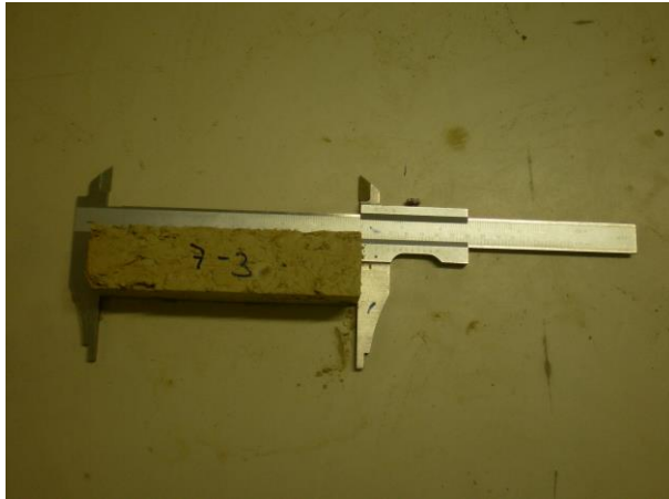
Fig. (2): Vernier scale for measuring the shrinkage The samples dimensions were measured with a vernier scale (Fig. 2).
