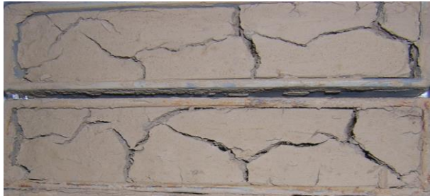
Fig. (4): Shrinkage and crack formation for earth bricks.
