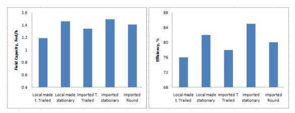
Fig (5) Field capacity and efficiency of locally made vs imported balers
