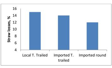
Fig (2) straw losses (unpicked straw) of the tractor pulled balers
