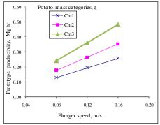
Fig. 6: Effect of different plunger speeds on the prototype productivity Mgh<sup>-1</sup> at mass categories of Diamond.
