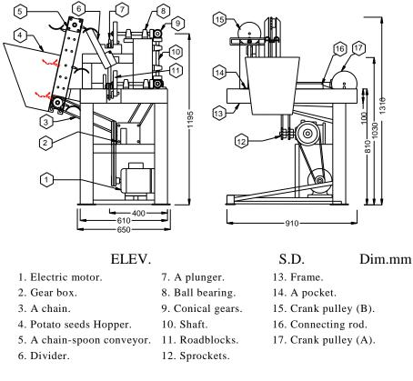
Fig. 1: Schematic diagram of potato cutting prototype.
