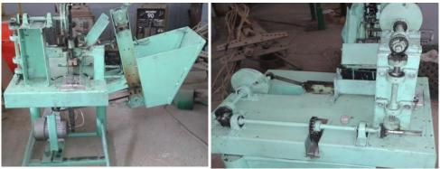
Elevation image. Side image. Fig. 2: Elevation and side images of potato cutting prototype.
