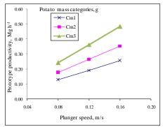
Fig. 5: Effect of different plunger speeds on the prototype productivity Mgh<sup>-1</sup> at mass categories of Sponta.
