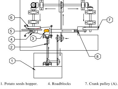
2. A chain-spoon conveyor.5. A plunger.8. Connecting rod.
