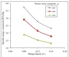
Fig. 12: Effect of different plunger speeds on the specific energy consumption, kWhMg<sup>-1</sup>at mass categories of Diamond
