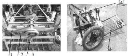
1- Frame 2- Digging blade 3- Separating 4- Transmission unit 5- Reciprocating link Figure (1): Digging harvesting components
