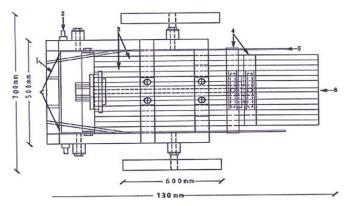
1- Share 2- Hatching points 3- Strips 4- Two longitudinal frames 5- Share frame 6- Separating unit Figure (2): Plane view of digging harvesting
