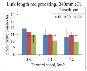
Figure (7): Harvesting forward speed via machine productivity
