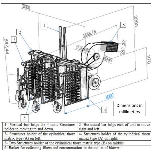
Figure 1: Prospective of the machine design in forward view.
