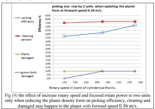
The main reason of this test is reduce stress of the engine of the machine to give more power to cylindrical thorns rotation. In Fig (9) shown the best efficiency than the other testes but low productivity to halve, because the dealing with one row at once. This test proves the success the idea of rotary cylindrical thorns matrix, but need to create the appropriate conditions of agricultures and Manufacturing of this design to improve machine performance.
