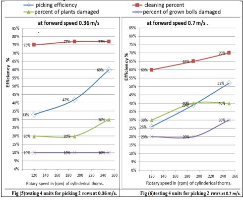
increased when increased the rotary speed of cylindrical thorn matrix because Probability of Collision between bolls and thorns was increased.
