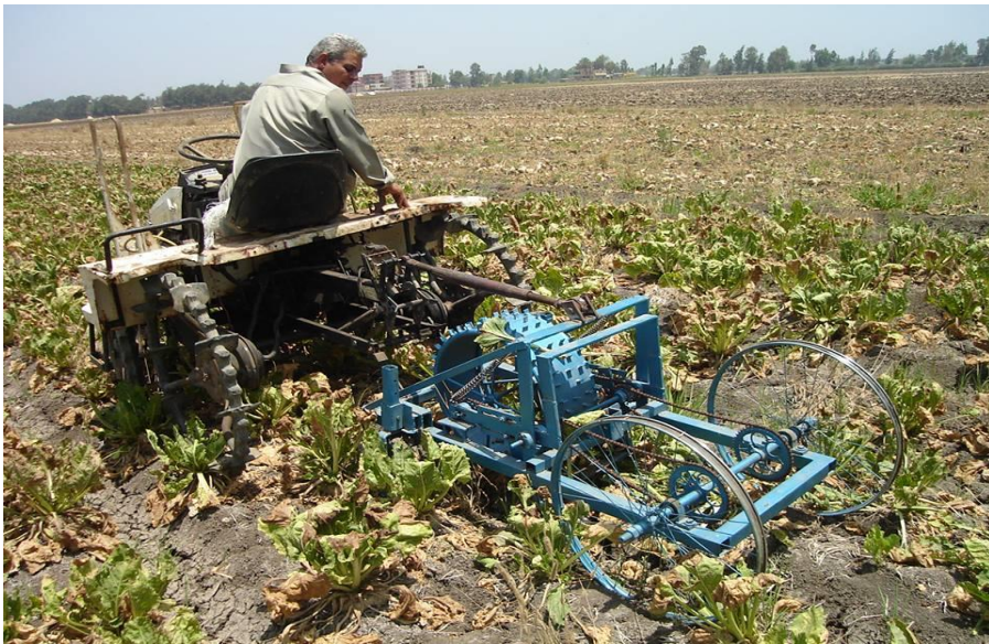
Fig.1: Prime mover of Yanmar ARP-8 Rice Transplanter and topper unit during operation.
