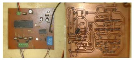
Figure (2): Control circuit for feeding seeds devices (stepper)
