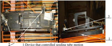
2- Control sensor, cut the electrical current
