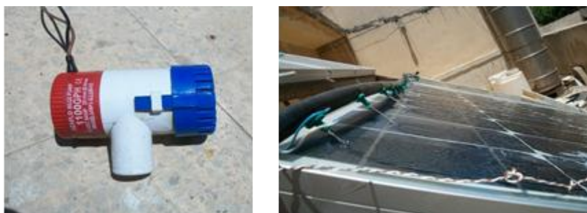
Fig. 3. DC Pump and water distribution hose with small water emitters
