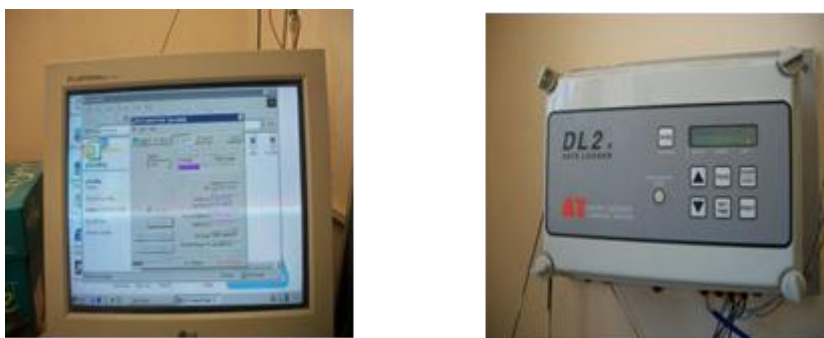
Fig. 4. Data logger DL2 version 5.0 connect with PC
