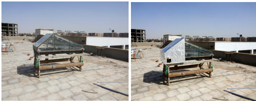
Fig. (1): Asymmetrical double-slope solar still with and without shading.
