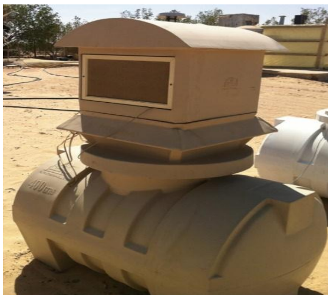
Fig. (16): Two identical water storage tanks; one equipped with fan and the other without fan.
