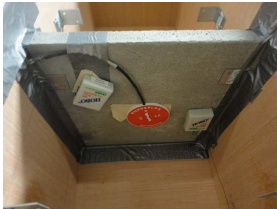
Fig. (7): Heat flux and temperature loggers attached to the specimen
