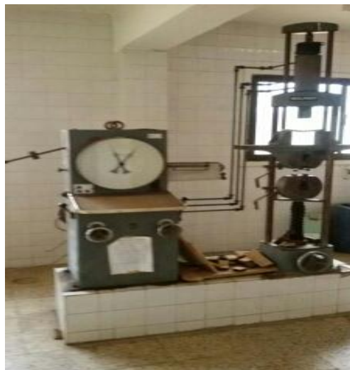
Fig. 2 the internal bond strength test machine in Tanta flax and oils Company
