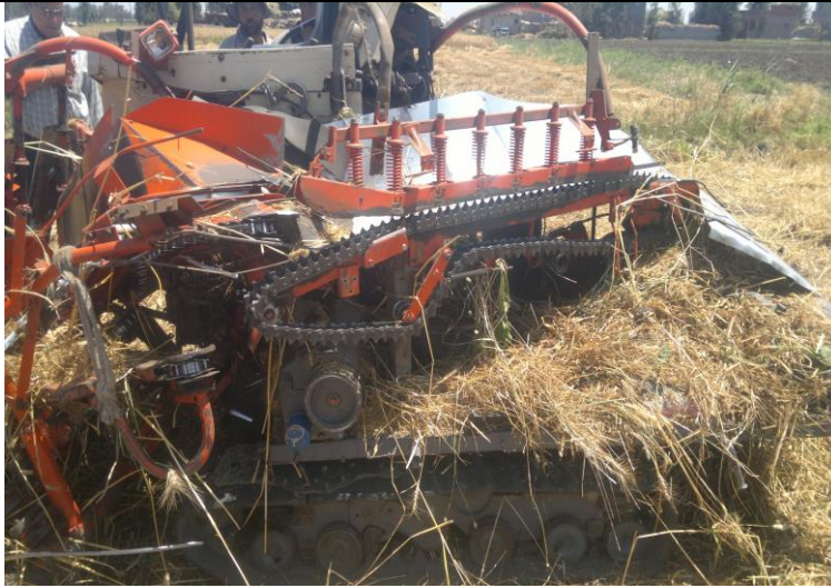
Fig. 1: Removing of threshing, winnowing and cleaning components and assembling a mat in site of them
