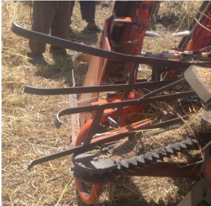
Fig. 3: Assembling repel arms on steering arm
