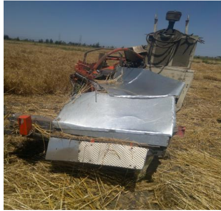
Fig. 4: Assembling a mat, under conveyer and a rear pile base
