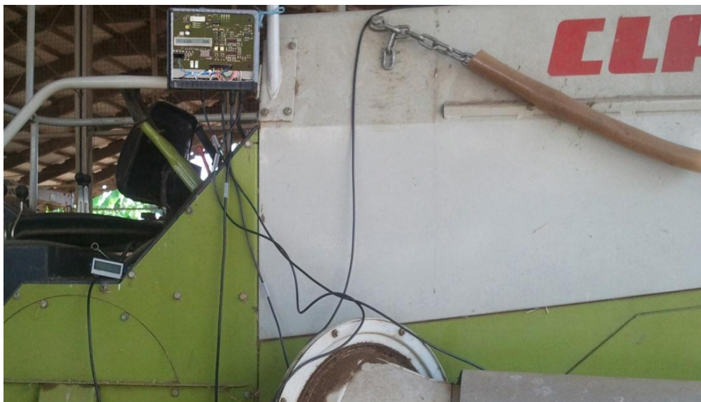
Fig. 5 Attaching fuel consumption device and extra display screen to Claas combine harvester for field testing
