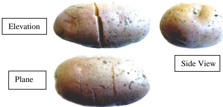
Figure (5) Cracked Potato Tubers in Three Directions After Force Deformation Test.
