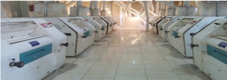
(Fig.11). The milling wheat machines (Break and reduction systems)
