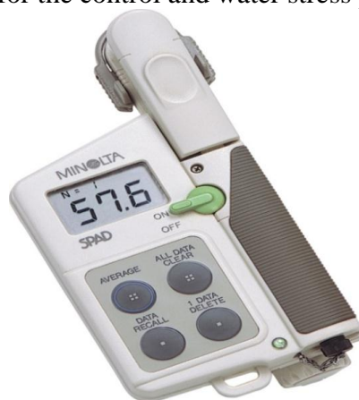
Fig. (2): Portable chlorophyll meter SPAD-502 for measuring chlorophyll in potato crop.
