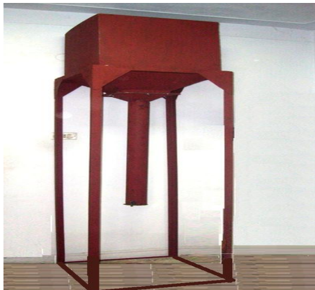
Figure (1): shown experiment set up to 8 cm diameter pipe with 1 m length and 90° vertical angle.
