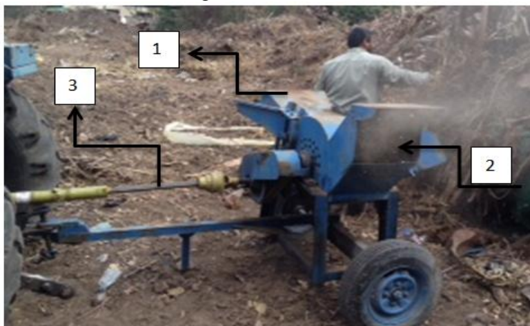
1- Open of in-let material 2- Out let gate 3- PTO connecting
