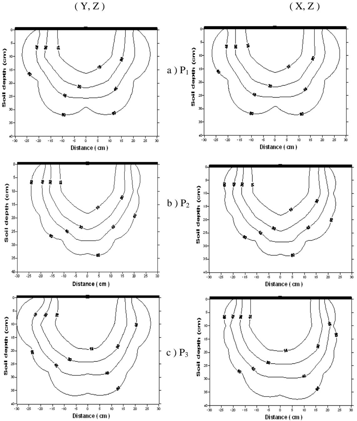
Figure ( 6 ) The water front distribution as a function of time ( min ) under different operating pressures in 2D diagram ( Y, Z ) and ( X, Z ).
