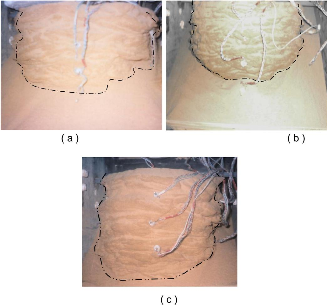
Figure (5) The wetted bulb produced in the soil box under different three operating pressures
