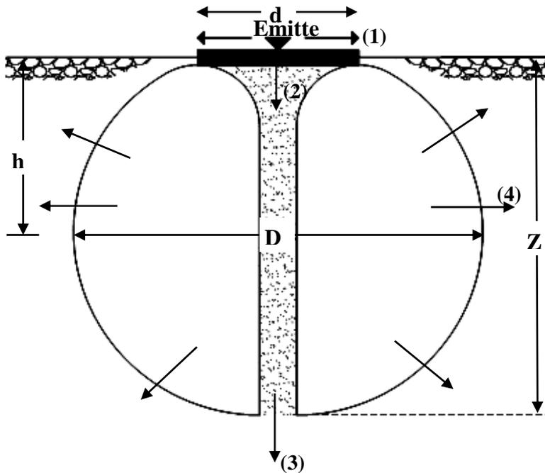
Figure (1) The dimensions of the wetted pattern (Zur (1999)) and driving force to water movement through wetted pattern (Rosenfeld (2000))
