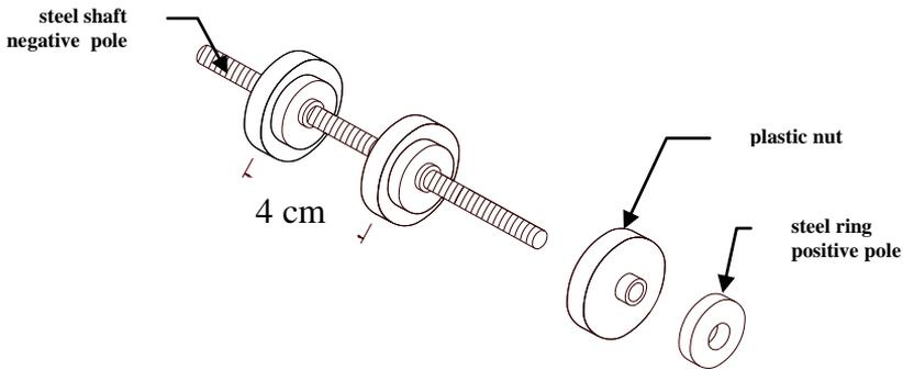
Figure (3) The measurement axis
