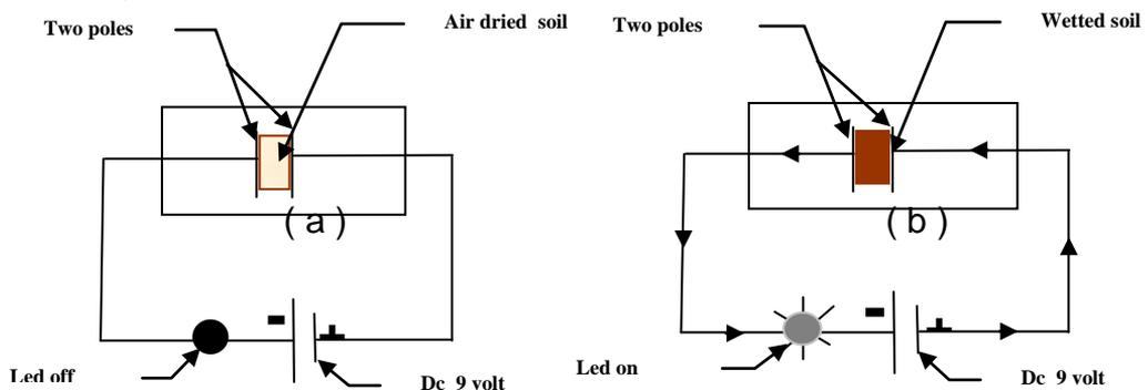
Figure (2) The electric circuit a) opened when soil dry
