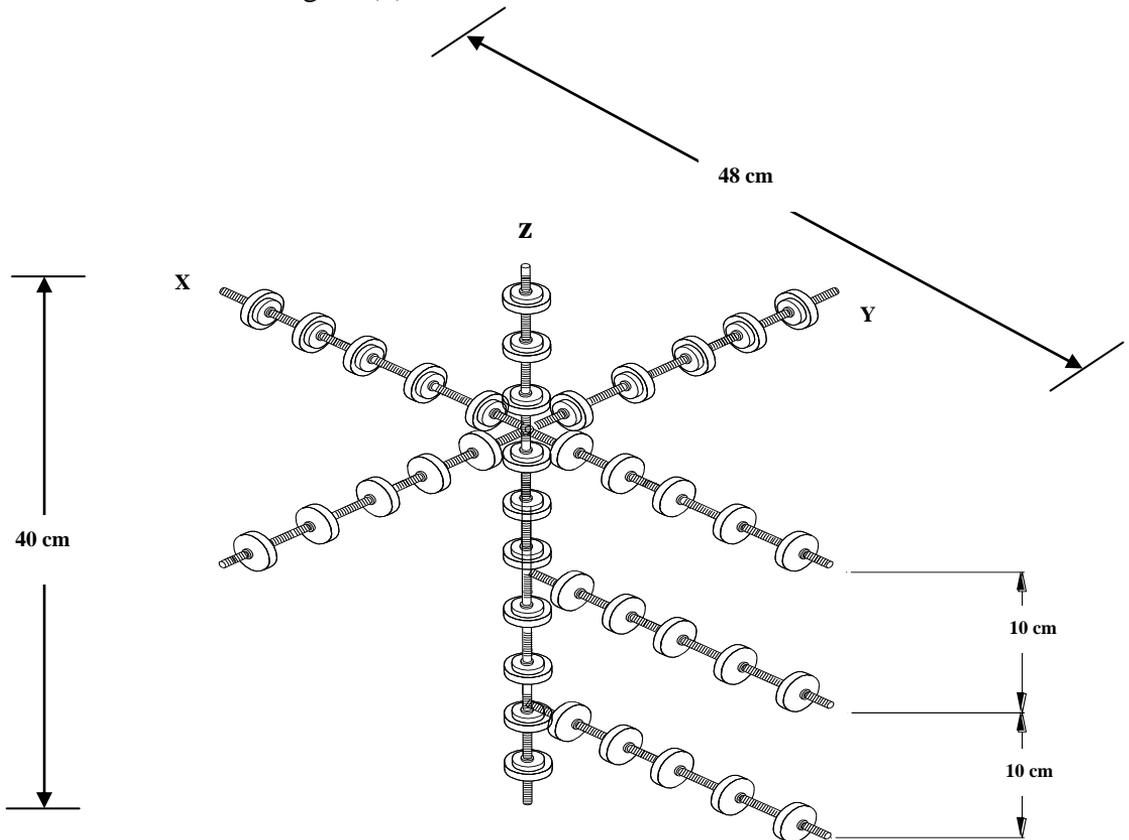
Figure (4) The measurement axes in three directions (Y, X, Z)
