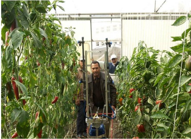
Figure 3: Evaluation of vertical boom site developed sprayer in piper crops under greenhouse conditions.
