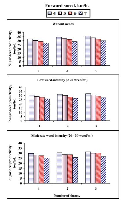
Fig. 6: Effect of forward speed, number shares on sugar-beet productivity without weed, at low and moderate weed intensity.
