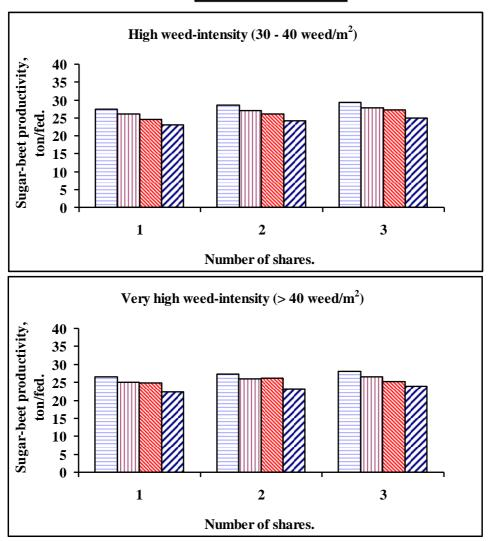
Fig. 7: Effect of forward speed, number shares on sugar-beet yield at high and very high weed intensity.
