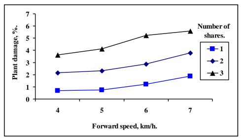
Fig. 5: Effect of forward speed, number shares on sugar-beet plant damage.
