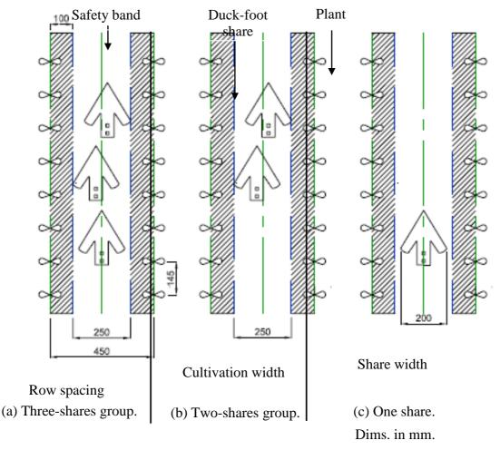
Fig. 2: Tested row spacing, intra-row spacing (plant spacing in the same row), number of shares, share width and safety-band width.
