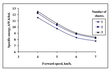
Fig. 8: Effect of forward speed and number of shares on specific energy.
