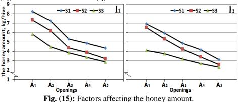
This is due to the improvement of hive conditions. It was noticed that the amount of honey increased with the ventilated, shaded and insulated hives according to the following descending order descending order  $(A_1 > A_2 > A_3 > A_4 > A_5)$ ,  $(S_1 > S_2 > S_3)$  and  $(I_1 > I_2)$ , respectively.
