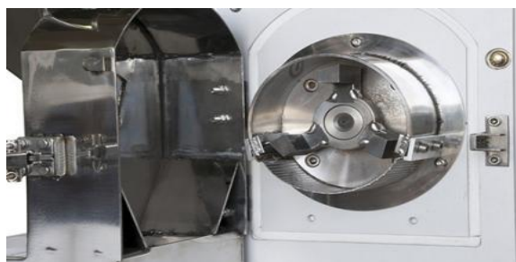
Fig.(2). Grinding chamber and blades for Hammer mill.
