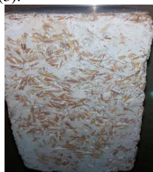
Fig. (4). Casted presume sample of Slag - Rice husk- Gypsum binder.
