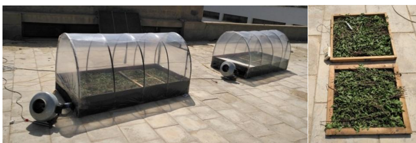
Fig. (2): Quonset shape greenhouse type solar dryer and traditional sun drying of mint
