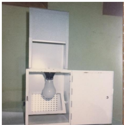
Fig.1: The reflection type crack meter
