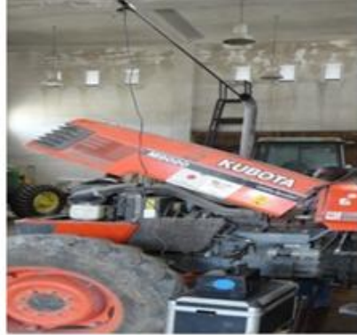
Fig.(3) The stack gas analyser connected to the tractor exhaust pipe
