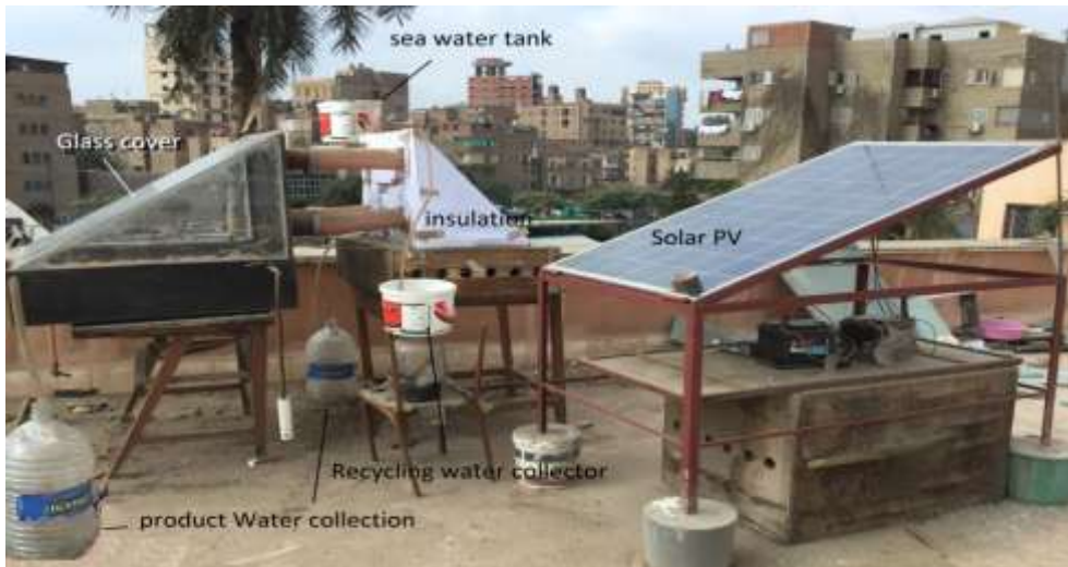
Fig. 2 (a) Photographic view of the overall experimental setup and the condensate water formation in stills
