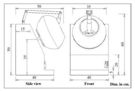
Fig. 1: Views of a seed-coating machine Abd-Al Fattah et al. (2015).
