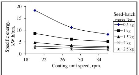
Fig. 9: Effect of coating-unit speed and maize seed batch mass on specific energy.
