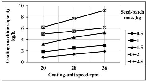
Fig. 6: Effect of coating-unit speed and maize seed batch mass on coatedseeds machine capacity.
