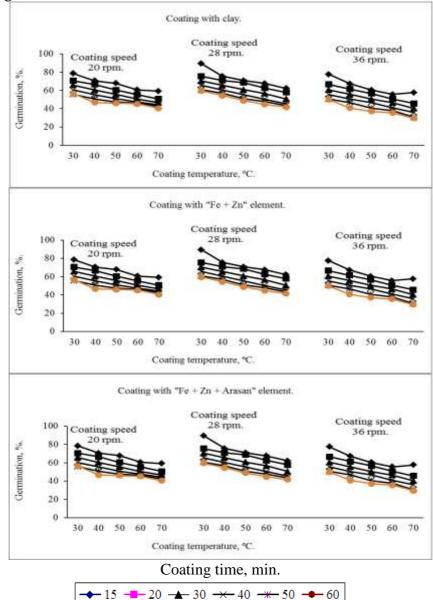
Fig. 5: Effect of coating temperature and time, by "Fe + Zn", "Fe + Zn + Arsan" and clay on the maize seeds germination and at constant seed batch mass of 2.5 kg. The germination of the maize corn-seeds without coating was 32.5 %.
