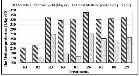
Fig. 2: The theoretical and actual methane production [*l*/kg vs]
