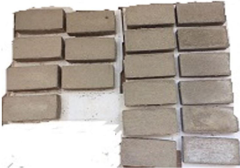
Fig. 2: Some of bricks manufacturing from the bagasse different ratios with cement kiln dust.
