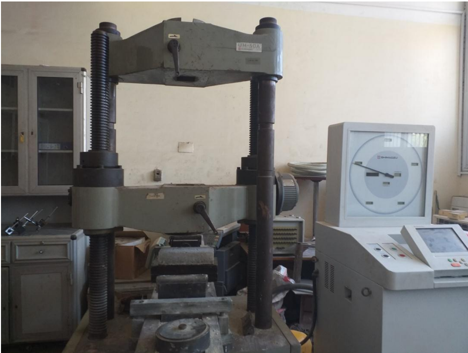
Fig. 3: Testing machine used for measuring compressive stress-strain and bending momentum.
