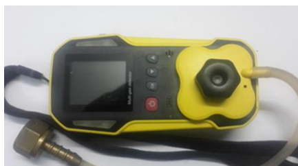
Fig.(2): The Biogas analyzer
