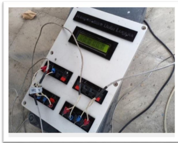
Fig. (3): Temperature data logger.
