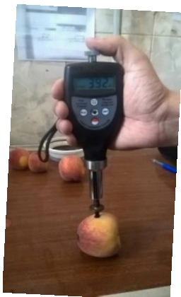
Figure 3. Fruit Hardness Tester, FHT-1122
