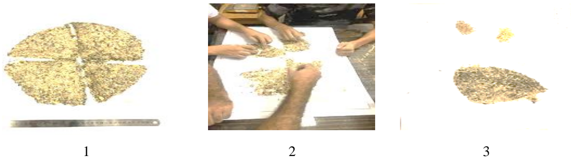
Fig. (5): Steps to calculate mixing efficiency
