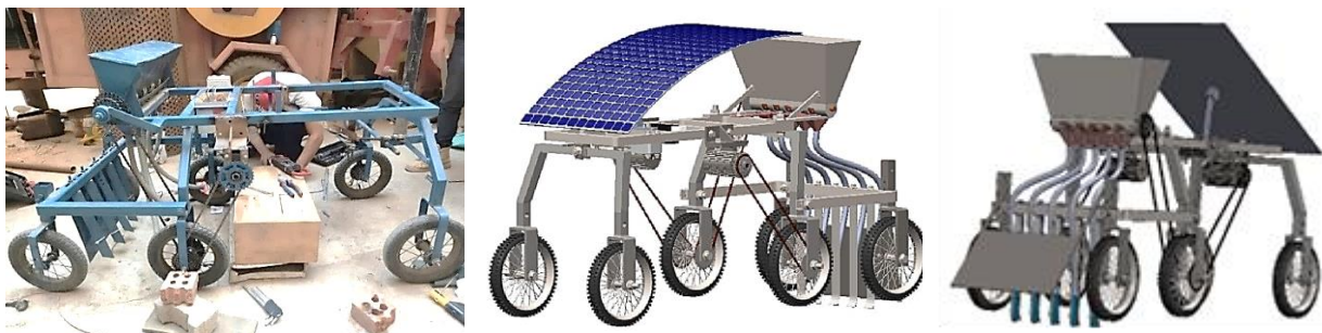
Fig. (1): Front view of the prototype solar-powered seed drill
