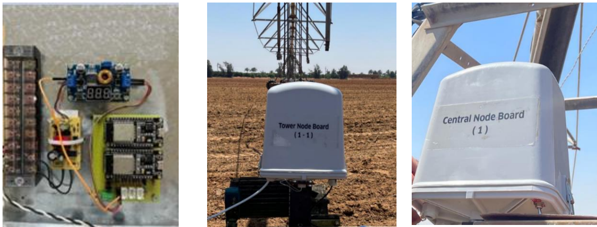
Figure (5): Components and position of Tower and central Node Board
