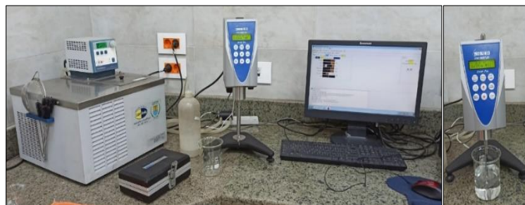
Fig. (3). Brookfield DV-II Pro Viscometer with a spindle (RV2)
