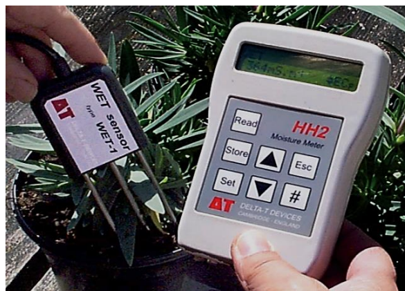
Figure (3): Model HH2 of the moisture meter device.
