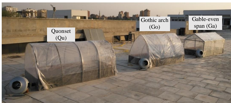
Fig (2): General view of the constructed greenhouse dryers
