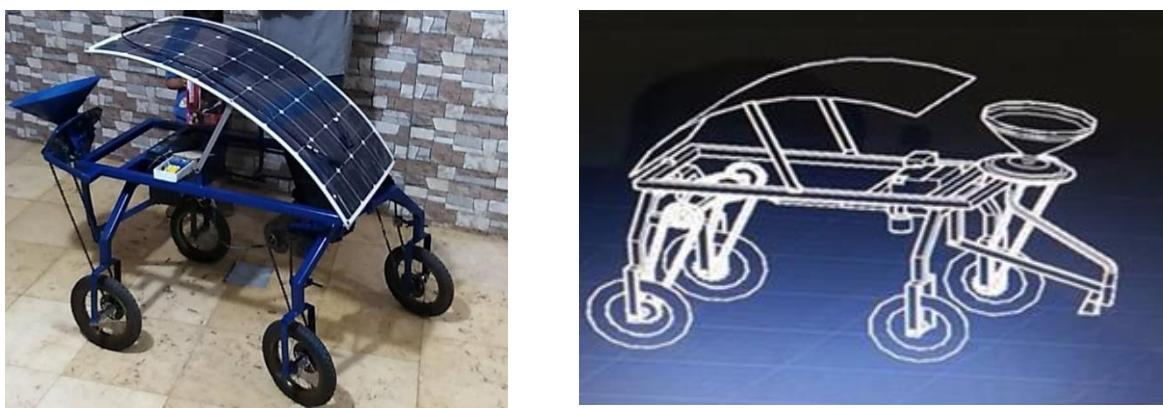
Fig. 2: The layout and main parts of developed spraying machine with solar photovoltaic
