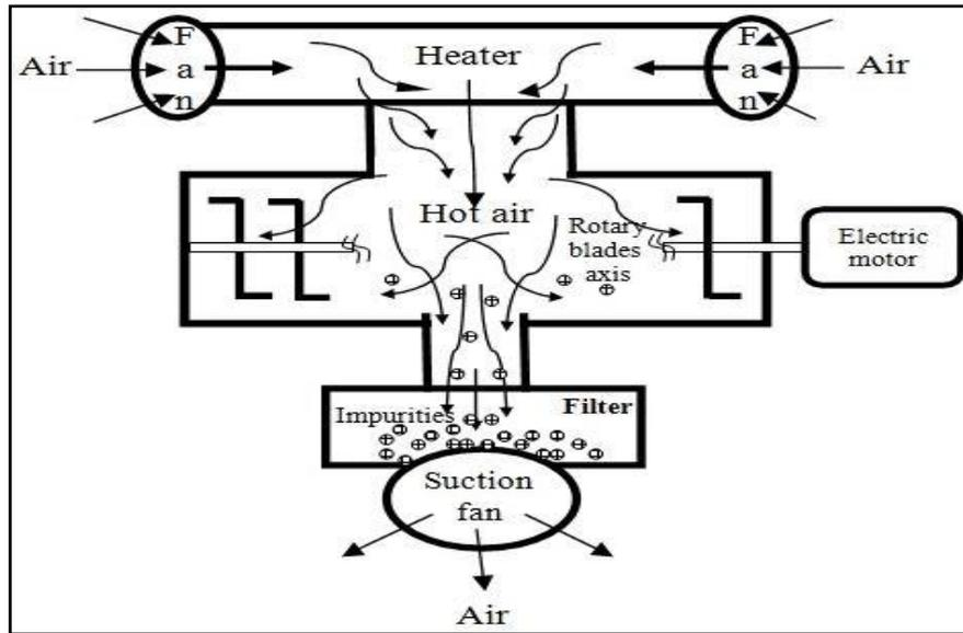
**Figure (4): A sketch diagram of sterilization and filtration cycles**
