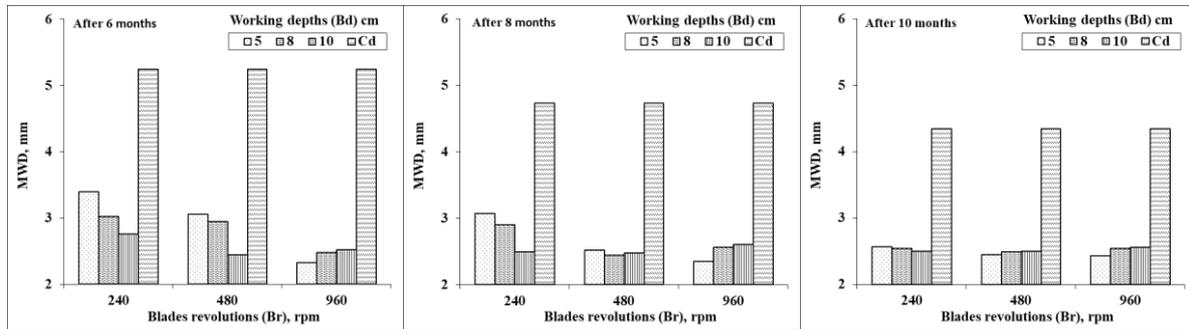
Figure (7): MWD for different working depths (Bd) and blades revolutions (Br) at different litter time periods (Mt).
