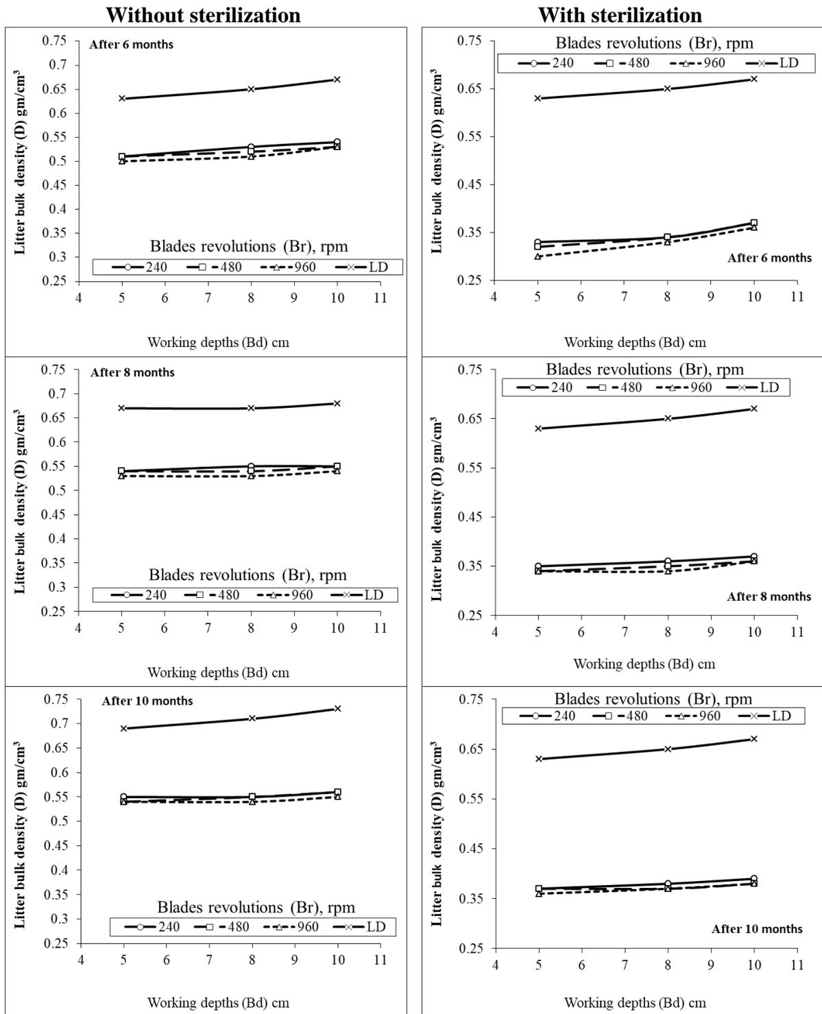
**Figure (5): Effect of working depth (Bd) on litter density (D) at different blades revolutions (Br) and different litter life period (Mt) under study, with or without sterilization process (St).**
