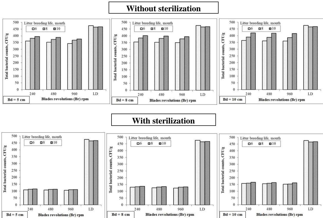
Figure (8) : Effect of rotary blades depths on total bacterial counts CFU/g at different blades revolutions (Br) and different litter life period (Mt) under study.
