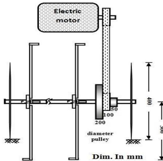
**Figure (2): main parts of flipping unit.**
